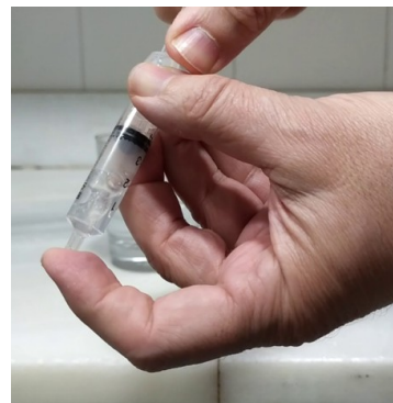
Fig. 11: At low pressure, water begins to boil at less than 100°C
